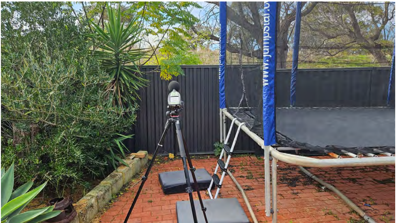
Figure 3-1: Photograph of Sound Level Meter on Site
