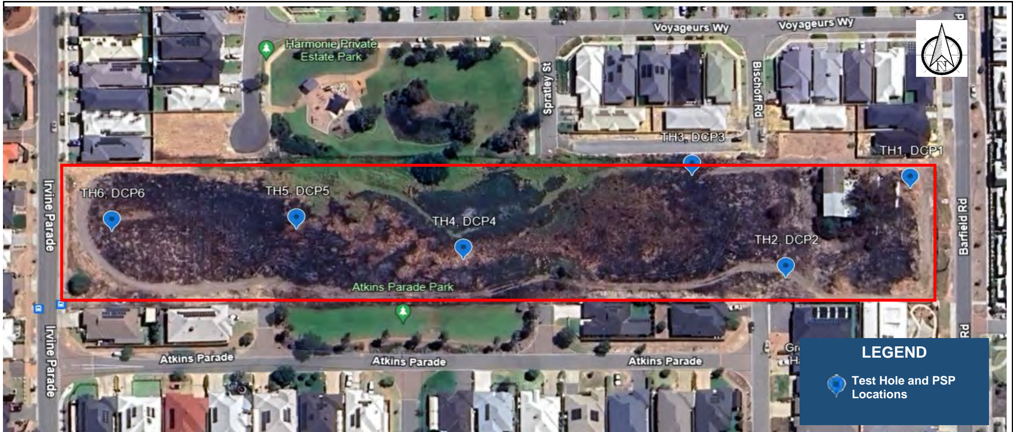
Site Sketch : Test Hole (TH) and Perth Sand Penetrometer (PSP) Test Locations
