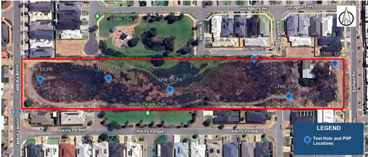
Figure 3 – Test Pit Locations – 116 Barfield Road, Hammond Park
