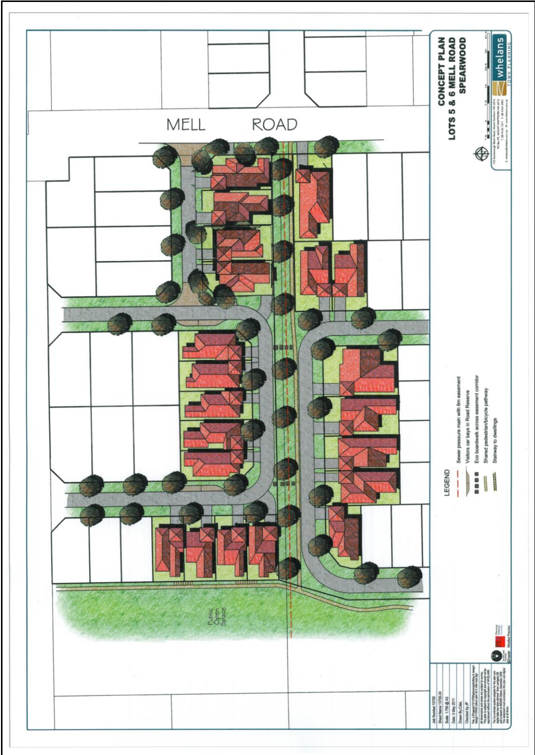
Figure 13. Concept plan Lots 5 & 6 Mell Road showing sewer corridor landscaped drainage swale and pedestrian accessway
